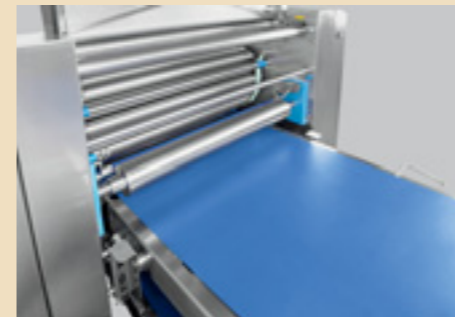
Only materials that can be easily cleaned are used. The conveyor belt in addition has sealed edges.
