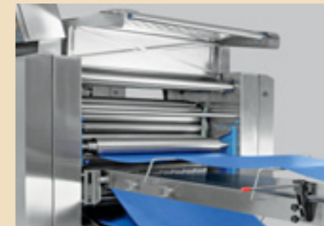
The wide-opening protective covers, the belt management system and the free spaces between the individual line components ensure good accessibility to all points where cleaning is required.
