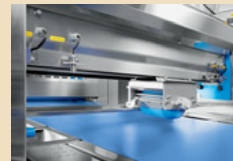
All parts of the ASTec line have been constructed in such a way that no materials can accumulate in niches or cavities.
