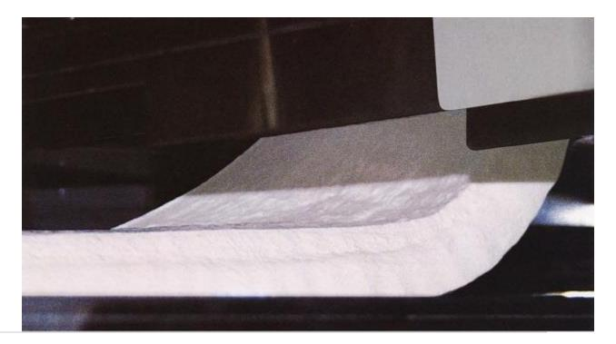
Forms dough blocks into a consistent dough sheet with the exact required output and transfers it to the next line.
