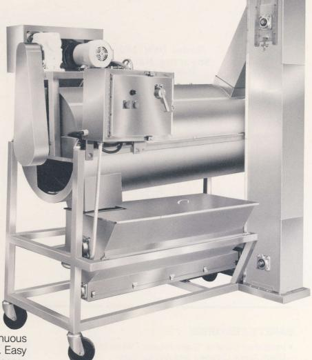
carries the sugar to the top of the drum where it is dropped through a perforated, rotating inner drum and onto the product flow. The donuts move through the sugar zone in a gentle turning, tumbling motion to the discharge opening. The speed of the sugar feed is easily adjustable to control the amount of coating on the donut. Loose sugar is continuously agitated and carried through the machine and the unused amount is automatically recaptured and returned to the sugar hopper.
