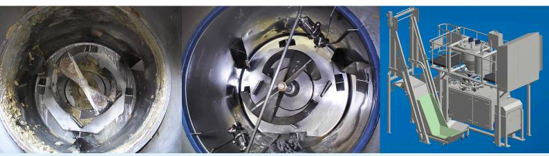
Patented CIP system The mixer is cleaned and rinsed out with a controlled small quantity of water
