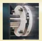
Uniquely designed shaft seals are sanitary and easy to remove.
