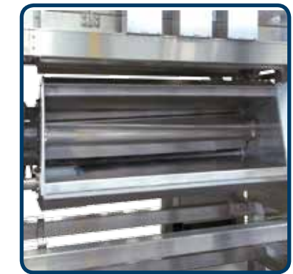
Kneading bowl with bowl/rotor tilting function forenhanced cleaning up to 180°
