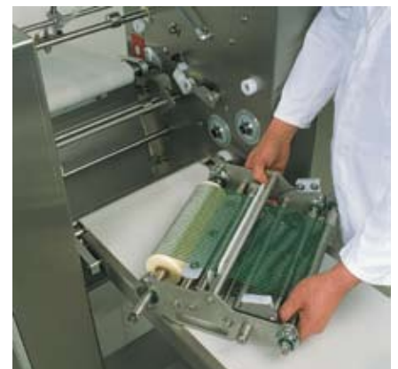
The coiling cassette can be completely removed for easy cleaning.
