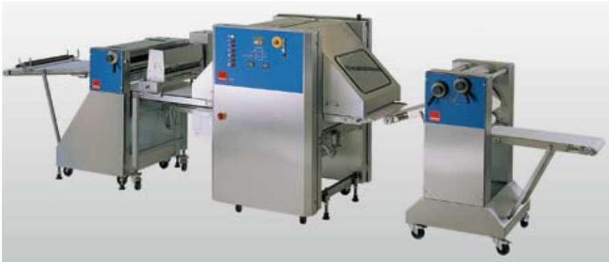
The CTR System with coiler for unfilled products (basic version).
