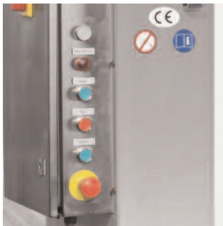
Pushbutton control for bowl elevators and tippers.
