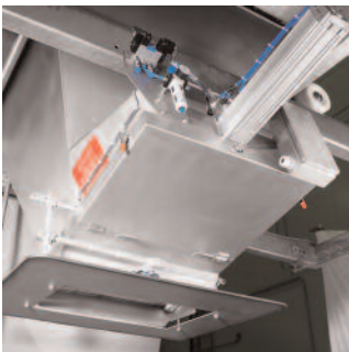
Funnel with pneumatic pusher to pre-apportion the dough.
