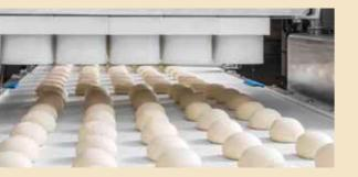
You produce perfectly round rolls with the RONDO Cup Rounder, the automatic round-moulding module, on both the RONDO Smart Bread Line and the ASTec
