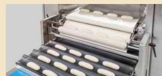
The RONDO long-moulding units automatically and reliably manufacture sandwich rolls and mini baguettes from dough pieces.
