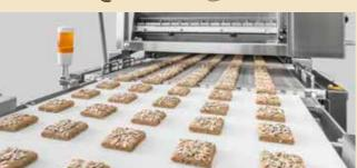
Refine your rolls with grains and seeds. RONDO depositors for coarse materials can sprinkle seeds on the top and underside of your rolls.
