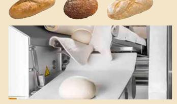
The RONDO BrotStar and other RONDO lines enable the automatic manufacture of long-moulded and round-moulded loaves of bread from wheat and ryemixed doughs.
