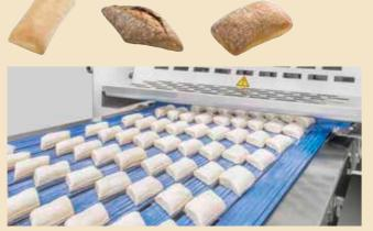
Whether square, diamond-shaped, triangular or rectangular – your rolls are accurately cut, separated and automatically panned onto the sheets.
