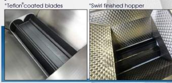
All types of non-stick finishes can be applied, and for real sticky doughs an oil spray sysyem can be outfitted.
