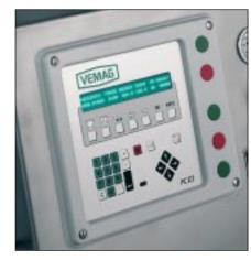
under their names. Set values are entered directly via the decimal keypad of the portioning computer and accepted with a single key. Weight corrections can be entered directly in grammes. All outputs are displayed in clear text in the desired language. The VEMAG Online net program package allows the portioning computer to be connected to one of the plant's master computers - and with a modem extension, to VEMAG Customer Service.
