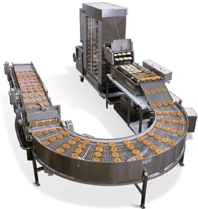
Century – Mark VI system with 180° curve conveyor, glazer, and cooling conveyor
