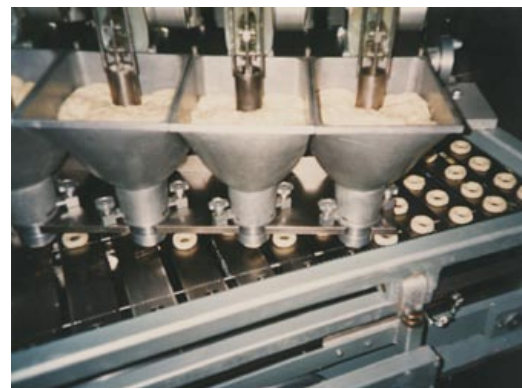
Belshaw Vacumatic – deposits ring donuts directly to automatic proofer
