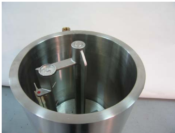
View of agitator with scrapers Easily removed for cleaning without tools
