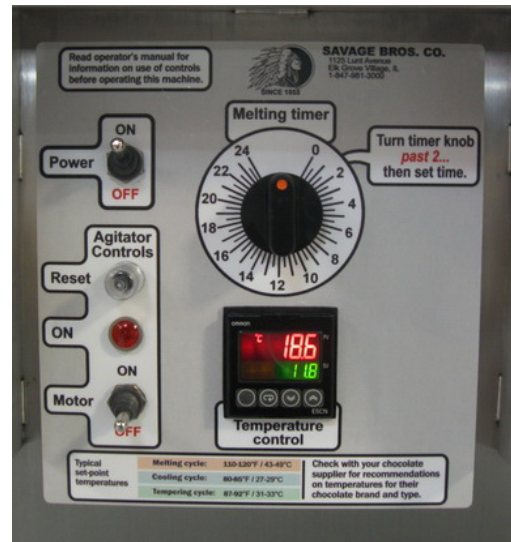
Control cover features 24 hour melt timer and digital temperature controller for accurate water jacket control
