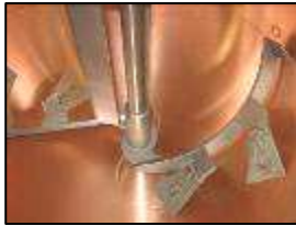
Warrior: Single-Action Agitator On Warrior model. Spring-loaded dairy metal scrapers on variable speed arm, with breaker bar.
