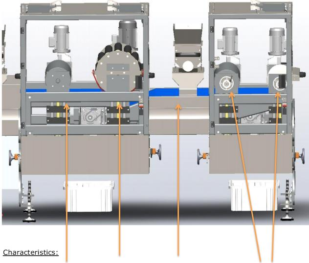
The first pressure roller of big diameter and **adjustable** to facilitate lamination.
