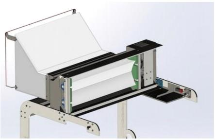
The hopper and the cutting system can be tilted **90 degrees** for easy cleaning.
