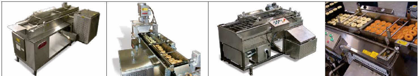
MODEL C6-8 — 6 ft. fryer, 2 standard donuts per pocket, shown with MD-2 cake donut depositor. C6-8 is electric only.
