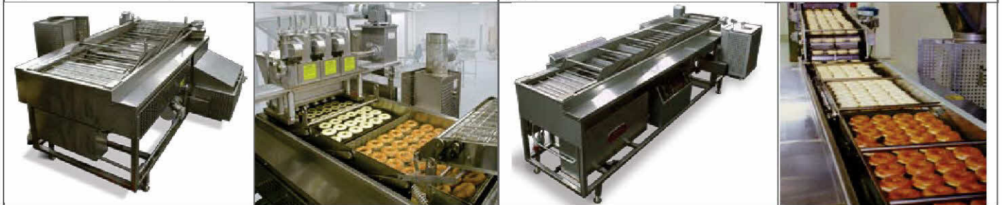
MODEL C6-24 — 6 ft. fryer, 6 standard donuts per pocket, shown at right with MDDRF-6 cake donut depositor. C6-24 is a gas-only fryer.
