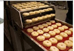
Transfer conveyor in operation
