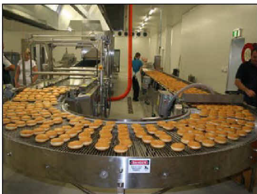
Above: Century system with 180° curve conveyor
