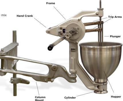
Belshaw Type B (photo also shows optional plunger, cylinder, and column mount)
