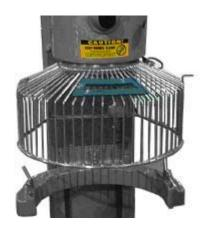
Push guard to the very top of the planetary and tighten. Place bowl into machine and lift to the upper limits to make sure the guard is in the correct position and has some clearance between the bowl and the quard.
