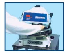
Once your desired time is set, pull down on handle and hold, applying pressure. The digital control will count down. A beeping sound will be heard when it reaches 0.
