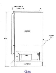
Water Requirements All Machines: 140 Degree Water - 84 GPH. at 20 PSI. MIN.
