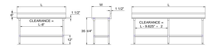
All units ship unassembled for reduced shipping cost. Units 7 ft. and larger are furnished with six legs. All dimensions are typical.
