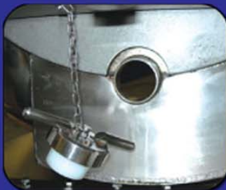
Screw off Drain Cap
