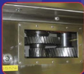
Oil bath gear drive with oil pump for long life
