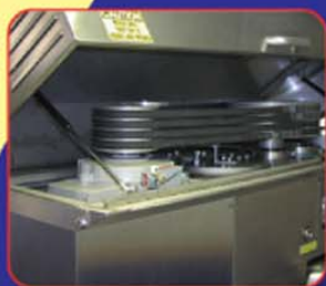
Hinged top cover for easy inspection and sanitation
