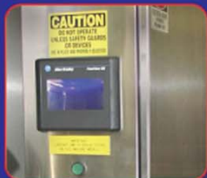
Fully programmable mixing using Allen Bradley PLC and Panel View
