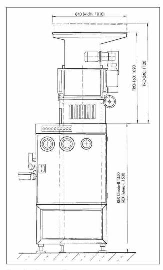
For easier cleaning or manual feeding the large dough hoppers TRÖ 160 and TRÖ 240 can be removed from the hopper with infeed rollers located underneath using a threaded spindle.
