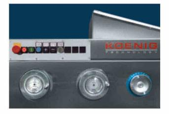
Clear and simple operation of the "STANDARD" execution. Dough weight and rounding speed adjustment as well as rounding height fine adjustment are carried out manually. The rounding time can be adjusted to different dough consistencies by means of a potentiometer.
