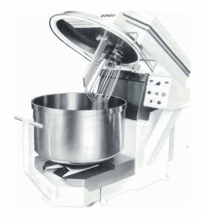
The "AV" Series also features a special bowl bottom and center bar which enable mixing of small batches. What's more, the SPI mixers are available in a "fix bowl" (F Series) version. And that's not all. An entire line of VMI Automatic Bowl Lifts complement these mixers to meet every production application.
