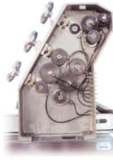
3-D Sheeting Head Drive Components and lubrication infeed lines.
